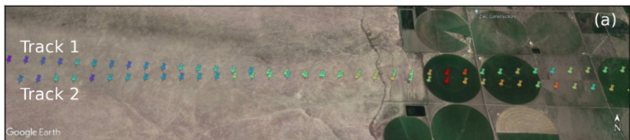
Figure 4.2.3d: HSRR obtained in two CYGNSS tracks across San Luis Valley in nearly coincident tracks and within two weeks difference. Features at scales much finer than the low sampling rate reflectivity are consistent between the two tracks. The low sampling rate reflectivity, not shown, only provided three points along each of these segments. From [P25].
